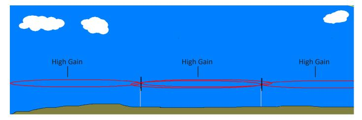
The above diagram visualises the use of high gain antennas utilised in a flat location **NOTE:** long thin beam width enabling RF communications between sites.
