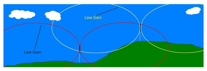
The above diagram demonstrates the correct antenna selection, here a low gain antenna is utilised at the telemetry site. **NOTE:** the wider beam width allows RF radiation to be directed in an upward direction and is able to reach to hill top above.
