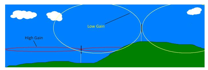
The above diagram demonstrates the effect of using a hi-gain antenna in a valley, **NOTE:** the beam with is narrow, and unable to reach the hilltop above.
