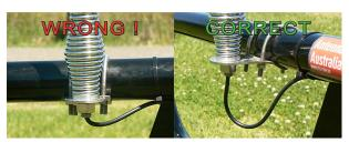
Route the RG58 low loss stranded cable carefully to your radio. Ensure that the cable is not stretched excessively and there are no sharp kinks.
