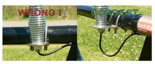
Important installation tip: Check the condition of your coaxial cable. Ensure a stress relief loop in the cable leaving the spring base. This will permit the antenna to flex in the usual manner during travel, without placing unnecessary tension on the cable.
