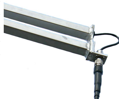
N-type female termination at rear of antenna
