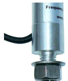
1/2"-12BSW threaded base with nut+washer, requires 12.7mm hole
