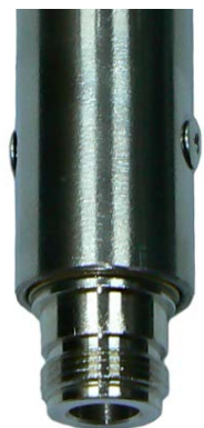
N-type female in base of mount section
