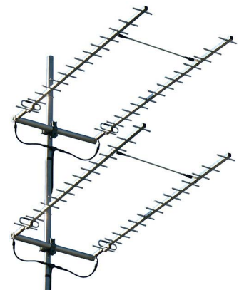
Horizontal polarised, horizontally bayed configuration
