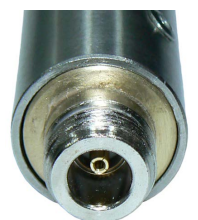
N-type female jack at base of mount section.
